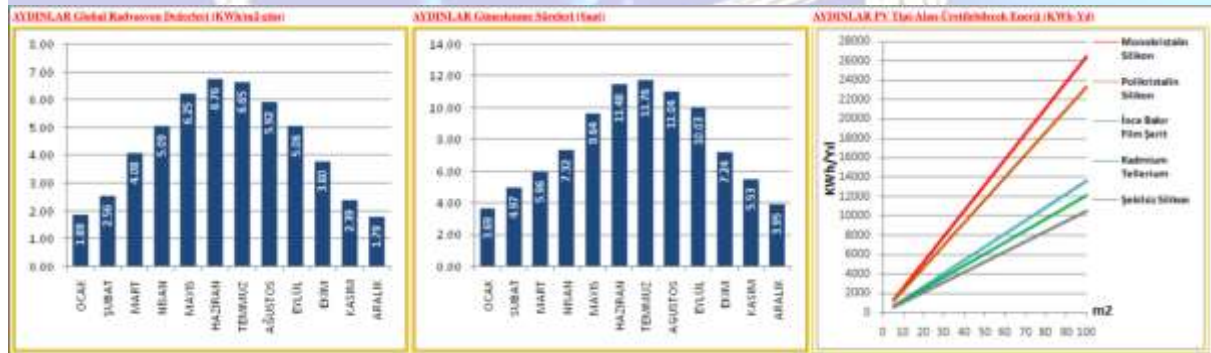
Graphic 1: a) Tillo District Radiation Values b) Tillo District Sunshine Duration c) PV Type -Area-Energy That Can Be Produced
